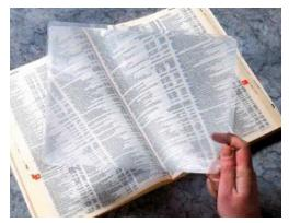
You can also find larger (much larger) ones in rear projection TVs. You can tell the ones that use Fresnel lenses because the image is only visible when you're directly in front of the TV and quickly disappears as you move off to the side.
