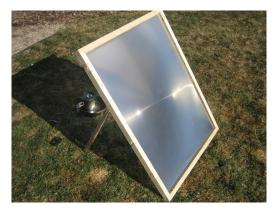
It focuses all of the light that hits the lens onto a 1" x 5" focal area. My digital thermometer maxes out at 500 degrees and when I line up the lens with the sun, it hits the 500 degree mark in just a few seconds on a clear day and will light a 2x4 faster than a lighter. According to research I've done, it will hit 1000-1100 degrees in optimal conditions.
