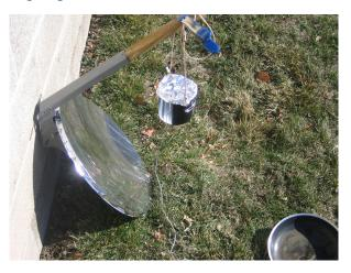
I've got a DirecTV dish. I stuck a small piece of wood out of the end of the mounting arm and hang my cup from it.
